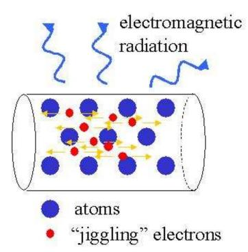
The "jiggling" of any charged particle emits radiation. Here, for example in a metal, alternating the voltage across the wire causes the electrons to move and the ions to remain motionless.
