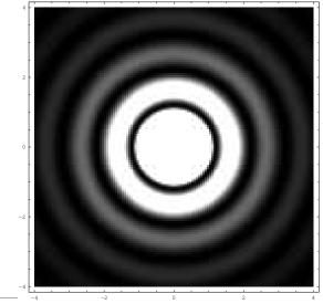
A point source emitting light at wavelength  $\lambda$ , as seen by a telescope of diameter D. The x and y axes measure angles in units of  $\lambda/D$  radians.
