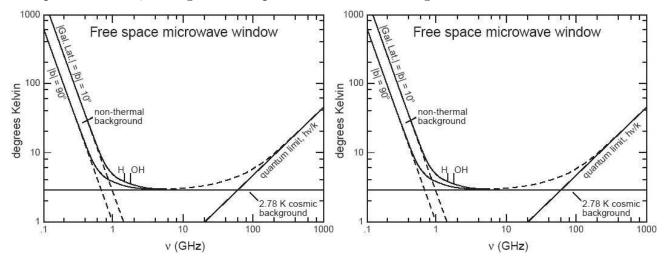
Diagram showing the effective noise temperature at various radio and infrared frequencies, from space (on left) and from Earth's surface (on right). The noise temperature is minimized about the "water hole" (resonant radio emissions from H<sub>2</sub> and OH<sup>-</sup>). Quantum noise, whose temperature  $T = h\nu/k_B$ , where  $k_B$  is Boltzmann's constant, only contributes to the higher frequencies in space. These plots are taken from Bernard M. Oliver, Acta Astronautica 6, 71 (1979).
